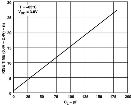
Figure 17. Typical Output Rise Time vs. Load Capacitance,  $C_L$  (at Maximum Ambient Operating Temperature)
