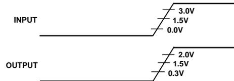
Figure 12. Voltage Reference Levels for AC Measurements (Except Output Enable/Disable)
