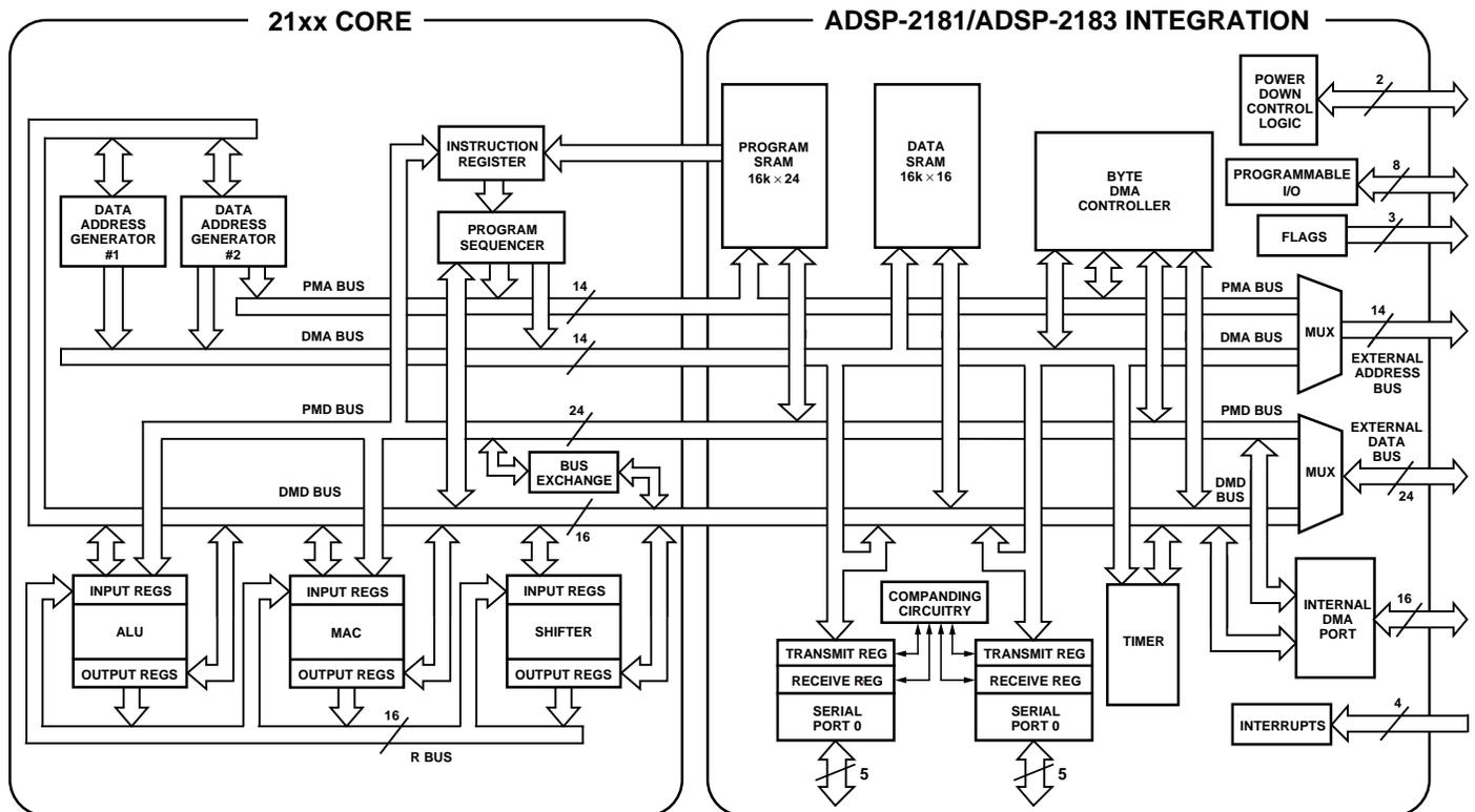
Figure 1. ADSP-2181/ADSP-2183 Block Diagram
