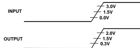
Figure 19. Voltage Reference Levels for AC Measurements (Except Output Enable/Disable)
