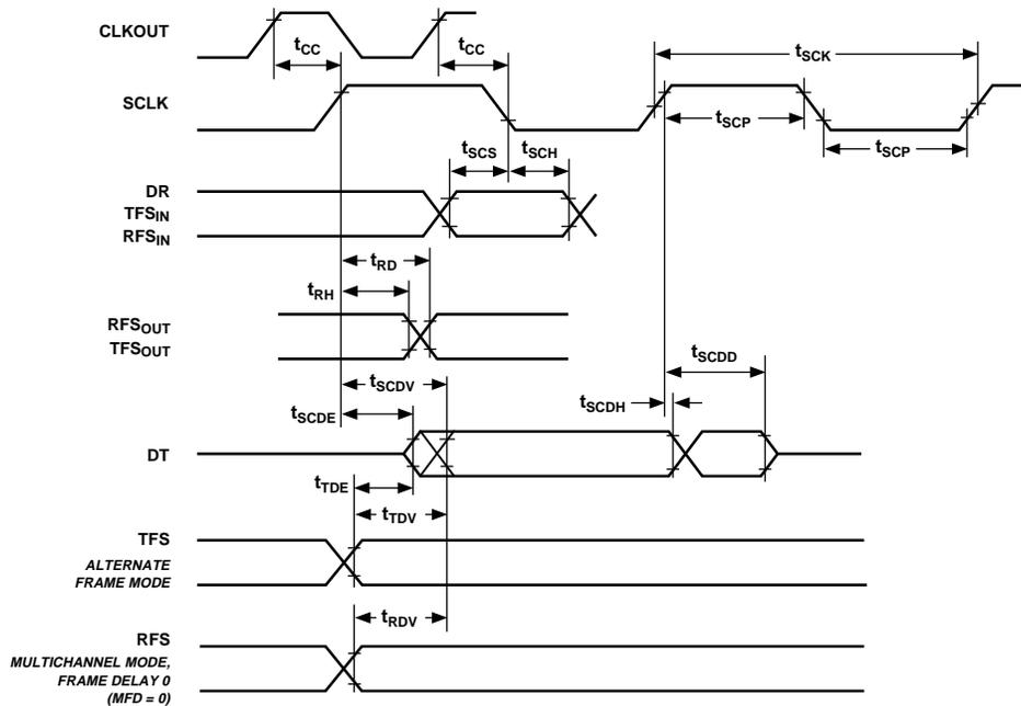
Figure 27. Serial Ports
