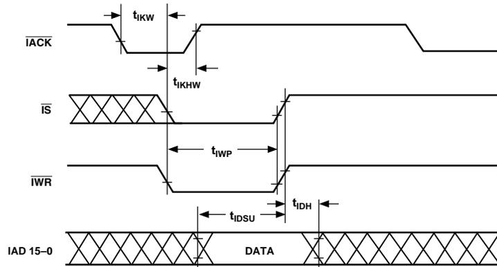
Figure 29. IDMA Write, Short Write Cycle
