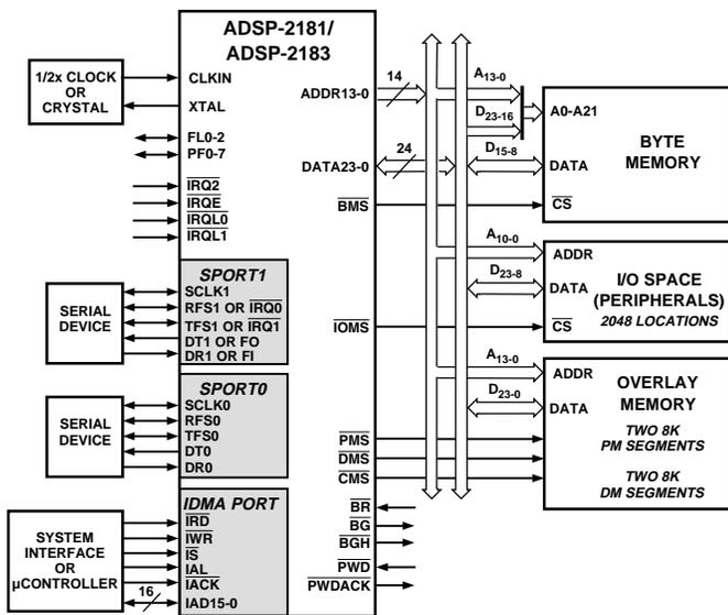
Figure 2. ADSP-2181/ADSP-2183 Basic System Configuration
